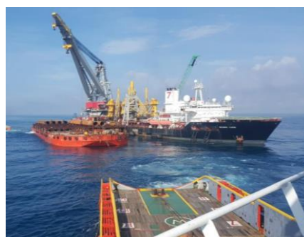
Marco Polo's MP Prospect supporting the installation of monopiles of the offshore wind farm construction in Taiwan
